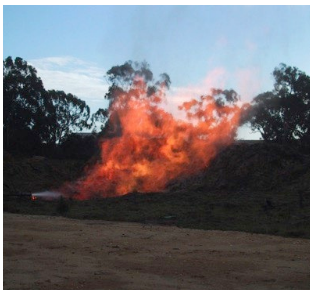
Figure 6: Flaring of Gas at Wombat-1 Gas Well
