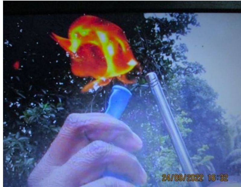
Field-test of gas bubbling from reservoir
