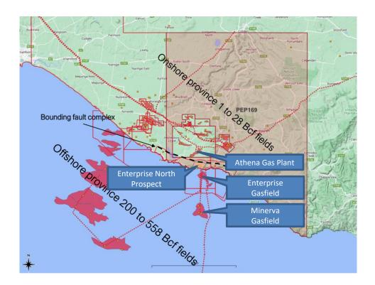
Cooper Energy operates the Athena Gas Plant, which was developed to process gas from the now-abandoned, offshore Minerva gas field. The Athena gas plant has spare capacity available.
